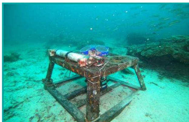
Exhibit 13: Acoustic Doppler Current Profiler over a period of time used to measure water current velocities (courtesy of INOS)
